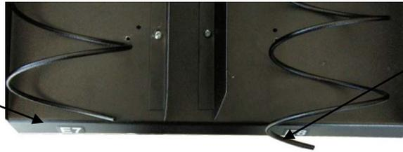
Improperly aligned Helix Coil
